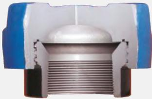
Recommended for air, water, oil, or gas service to 2,000 PSI NSCWP. A blanking cap with Buna-N 'O' ring seal provides an efficient and dependable closure. The threaded sub is interchangeable with Fig. 200 threaded sub. Also available with butt weld ends.
