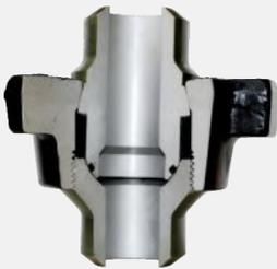
Recommended for high pressure manifolding and drilling rig use where alignment of piping components is a problem. Recommended for air, water, oil, gas or mud service to 10,000 PSI NSCWP. This union has a ball seat that allows a total of 15° (±7 1/2°) angular adjustment. An 'O' ring seal in addition to the metal-to-metal seat assures a pressure tight connection.
