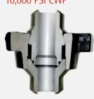
Recommended for high pressure manifolding and drilling rig use where alignment of piping components is a problem. Recommended for air, water, oil, gas or mud service to 10,000 PSI NSCWP. This union has a ball seat that allows a total of 15° (±7½°) angular adjustment. An 'O' ring seal in addition to the metal-to-metal seat assures a pressure tight connection.
