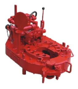
Sara Tongs are available in a variety of models, sizes and types to handle casings, drill collars, sucker rods and tubing including chrome tubulars and can be supplied with hydraulic or manual backup assemblies.
